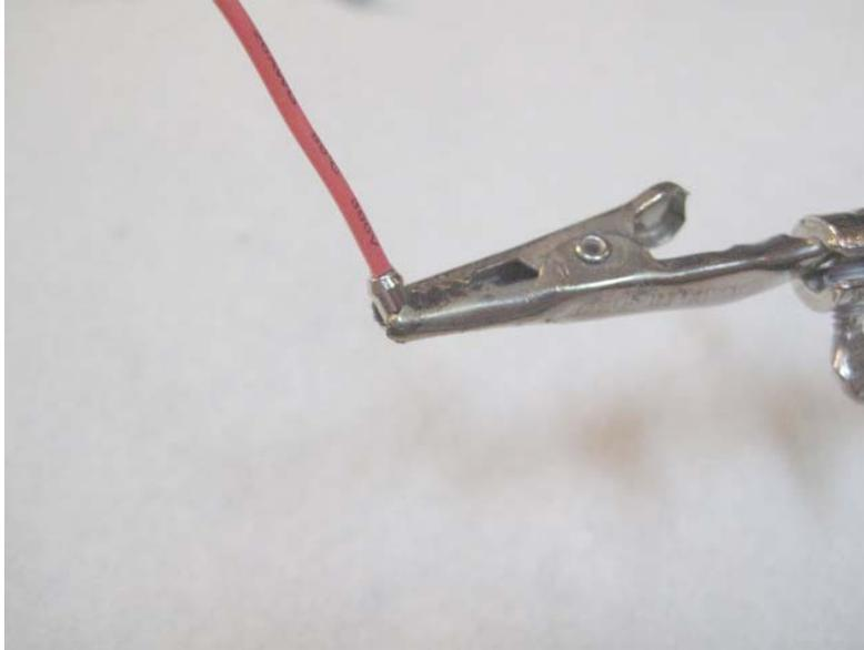
C. Wire a 20g black wire to the inside wall of the underside of the connector. It helps to first scruff up the area to be soldered on the connector, then apply flux, then apply a dab of solder.
